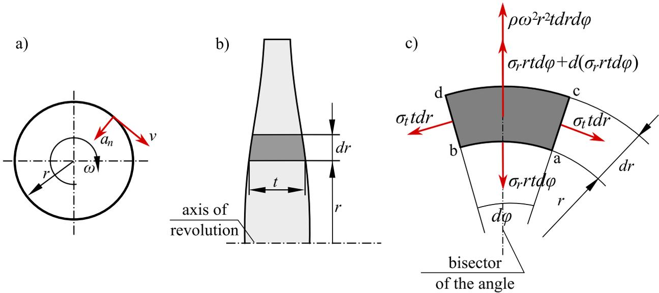
Fig. 1. Rotating disk: a) given parameters; b) radial section c) force distribution
