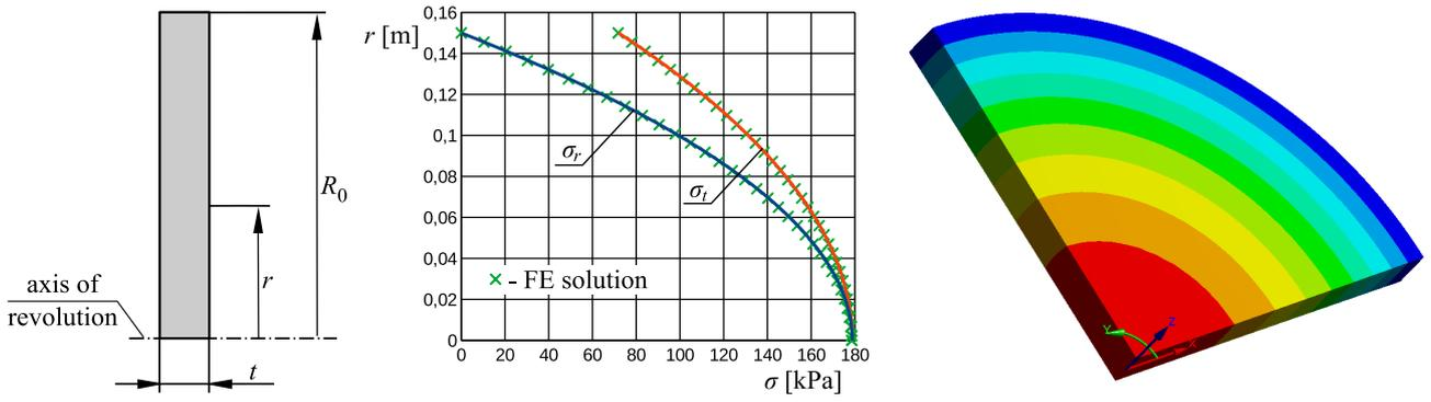
Fig. 3. Stress analysis in the rotating disk with constant thickness: a) geometry; b) stress distribution; c) view of the finite element solution
