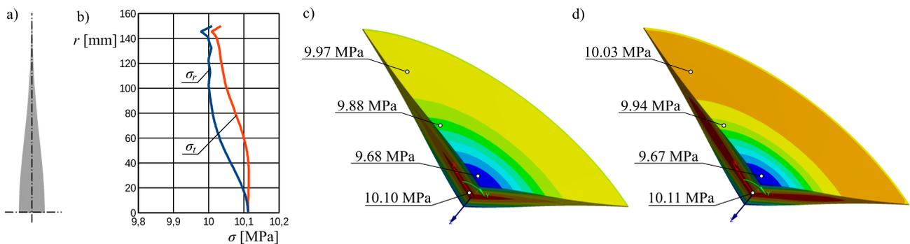
Fig. 5. Stress analysis in the rotating disk: a) geometry; b) stress distribution in the symmetry plane; c) radial stress; d) hoop stress
