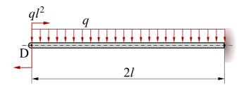
c) determine the vertical displacement and the slope at point D
