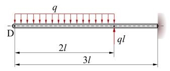
d) determine the reaction at point D
