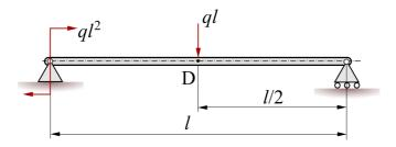
b) determine the slope (angle of rotation) at point D
